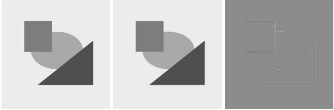
Figure 3.5: From left to right: initial geometric image f , \tilde{u} , \tilde{v} + 150 , computed with Db3 in the translation invariant setting, \alpha = 0.5 , \gamma = 0.01 .
