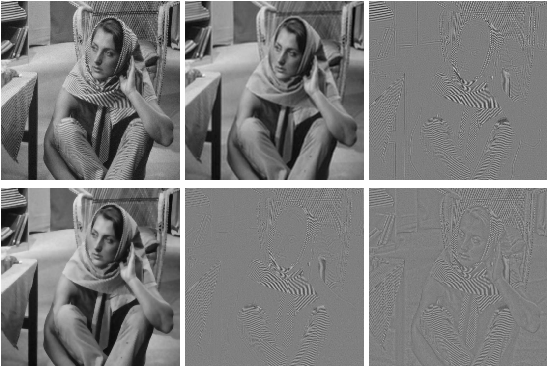
Figure 3.9: Top from left to right: initial woman image f , \tilde{u} and \tilde{v} + 150 , computed with Db10 (Method C), \alpha = 0.5 , \gamma = 0.002 ; bottom from left to right: u and v obtained by the Vese–Osher TV model and the v component obtained by the Vese–Solé–Osher H^{-1} model.
