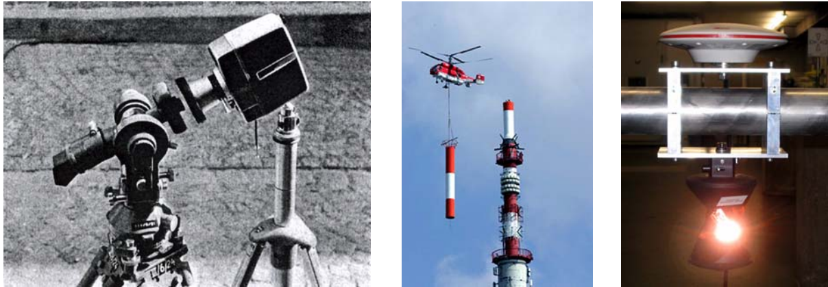
Fig. 2: Geodetic progress in Olympic Tower Monitoring: (a) Theodolite Wild T2 combined with a Nizo S8 film-camera in 1972, (b) change of the TV-antenna with a helicopter and (c) installation of a GPS-antenna and a 360° prism in 2005.
